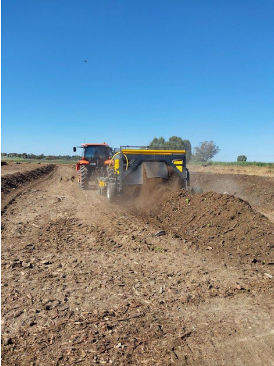
Windrowing the FOGO material
